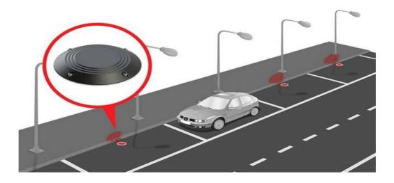
**Identification between Animals and Vehicle**:-It may happen that the light may light up if any animal passes over the sensor so a method of prediction based on the speed of movement will be enabled which will calculate the speed and depending on that the light will lighten up and in addition to that error will be less as vehicle have greater surface area and hence have higher probability of triggering the sensors.
