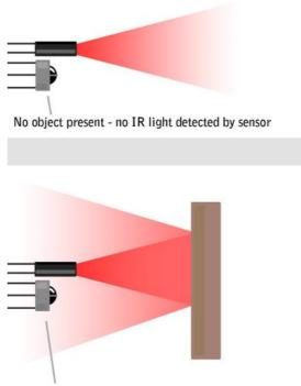
Object present - reflected IR light detected by sensor
